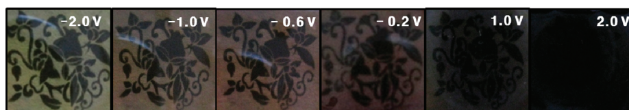
Figure 4. Photographs of electrochromic switching in one cell (RGBY) taken after placing the ECD on a white paper background with black bouquet, at different potentials in two electrodes with liquid electrolyte.
